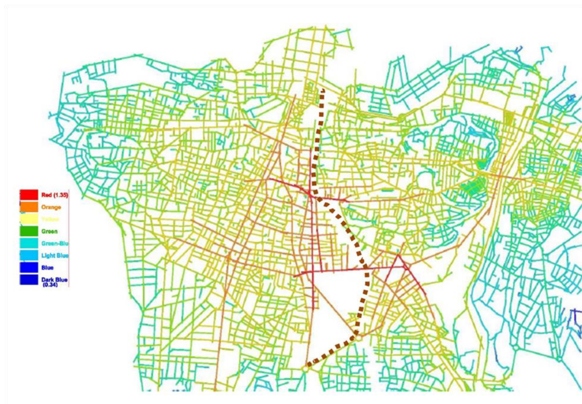
Fig. 1 Axial Map of Beirut Indicating the disconnection between east and west along the demarcation line (red dotted line) and impact on connectivity of the network: red being highest, and blue being lowest connectivity (Source: by Author)
