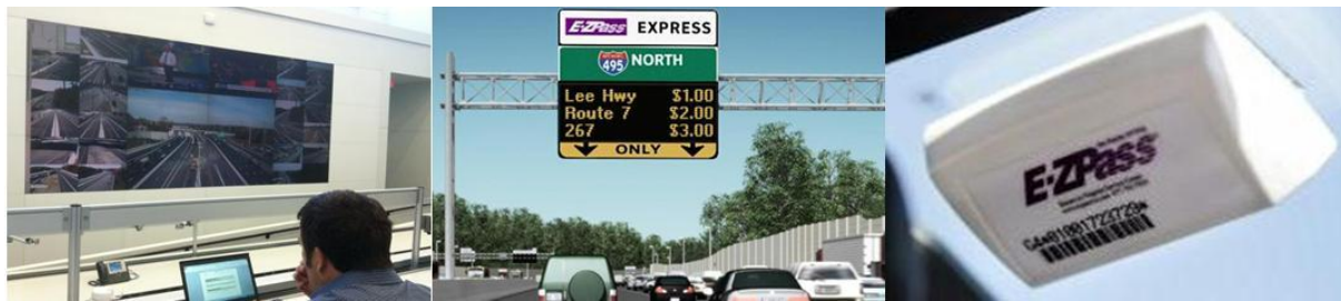
Fig. 4: Congestion pricing: Control panel, fares display chart and in-vehicle collecting fare system (Source: Virginia Department of Transport VDOT Express Lanes System)
